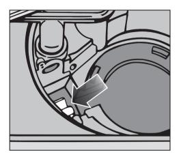
The drain pump is situated under the non-return valve (see arrow).
